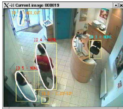
Figure 5. Ellipsoid masks of detected persons on the real image (highlighted ellipses)
