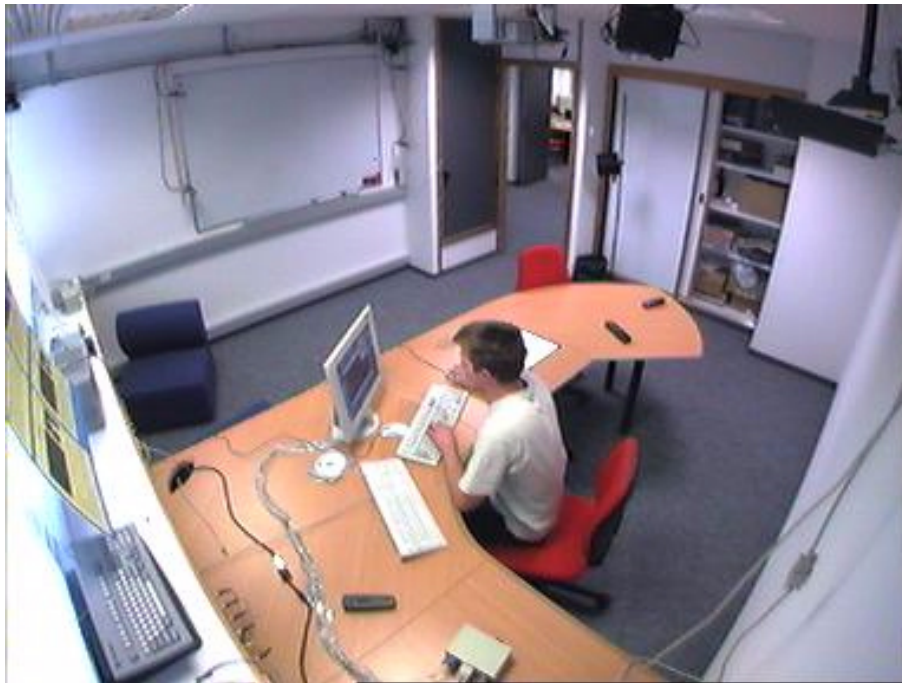
Figure 5. The augmented meeting environment is an office environment equipped with a microphone array, wireless lapel microphones, a wide angle surveillance camera, five steerable cameras, and three video-interaction devices.
