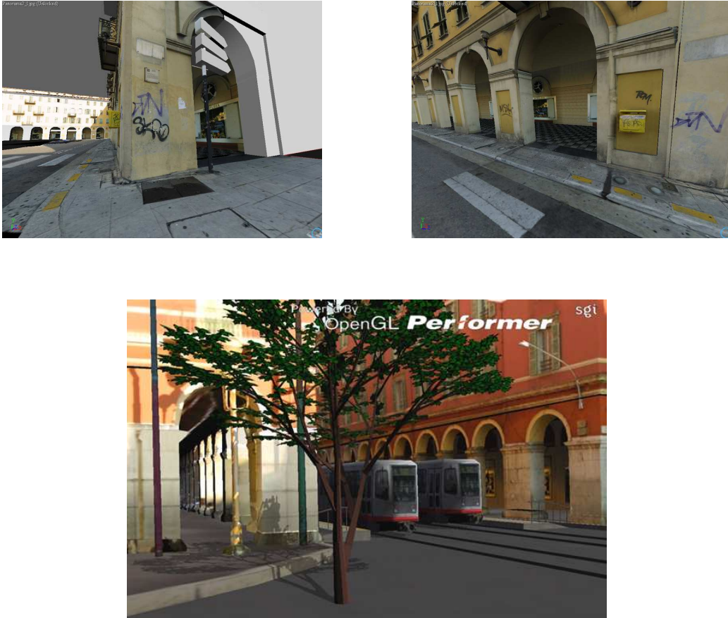
Figure 15. Above, partially textured reconstruction of Garibaldi square, developed for the CREATE project, and below an image of the CAVELib simulator showing our virtual environment enhancements (point-based rendering for vegetation, shadows and view-dependent texture mapping), integrated into a VE platform. The simulation also include 3D sound.
