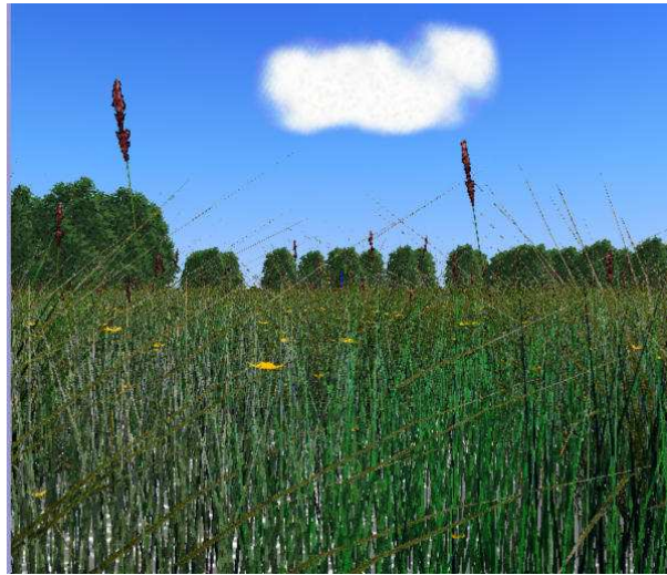
Figure 1. Plausible rendering of an outdoors scene containing points, lines and polygons [18], representing a scene with trees, grass and flowers. We can achieve 7-8 frames per second compared to tens of seconds per image using standard polygonal rendering.
