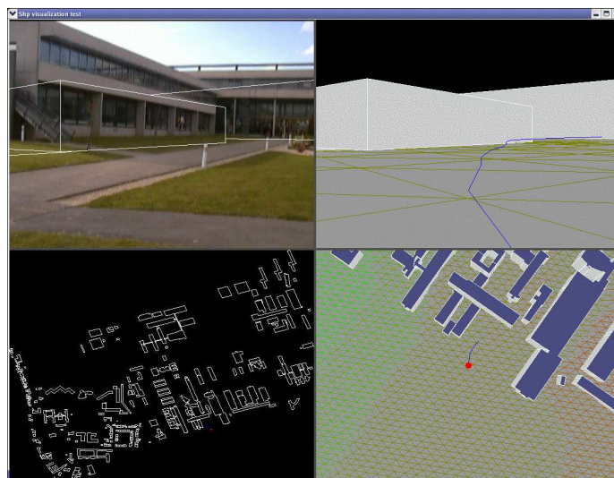
Figure 4. (a)- acquired video with superimposed GIS data; (b)- rendered GIS data with camera path in blue ; (c)- global map of GIS data, with camera path in blue and current camera position in red ; (d)- zoom on the GIS data and camera path around the current camera position.
