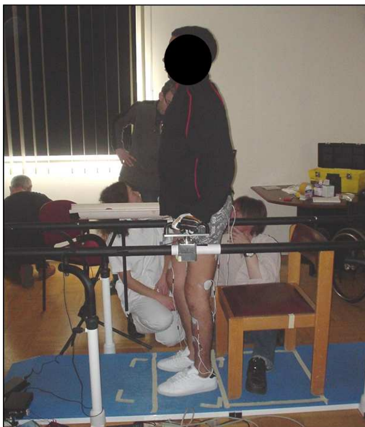
Figure 7. Experimental setup with the VICON, force sensors on both handles and sensitive insoles.
