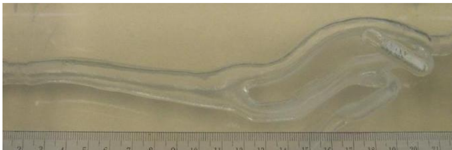
Figure 2. Phantom built by rapid prototyping from the surface mesh of the computational model of the carotid artery network.
