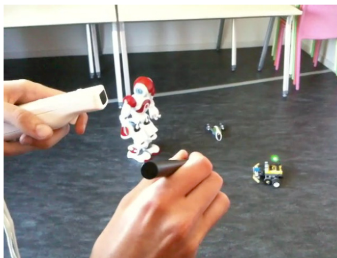
Figure 2. By using a Wii mote and a laser pointer we can easily interact with a robot and show it objects.
