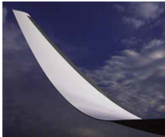
Figure 3. Winglets improve efficiency of fixed-wing aircraft.
