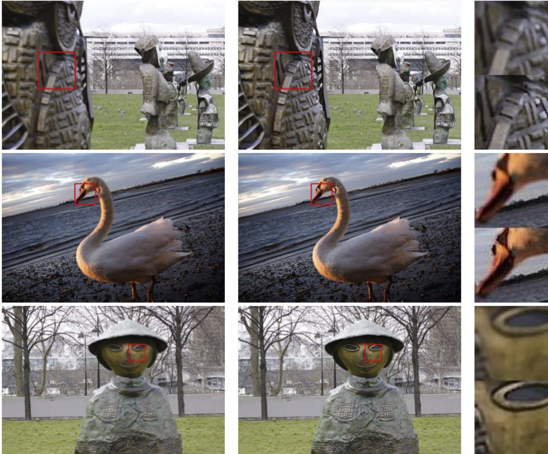
Figure 5. Sample deblurring results on real images. From left to right: blurry image, deblurred image, close-up corresponding to the boxes shown in red. Note that our estimated deblurred image has more detail.
