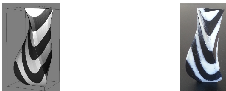
Figure 1. Left. A two-colored vase is modeled in IceSL. Right. An early printed result.
