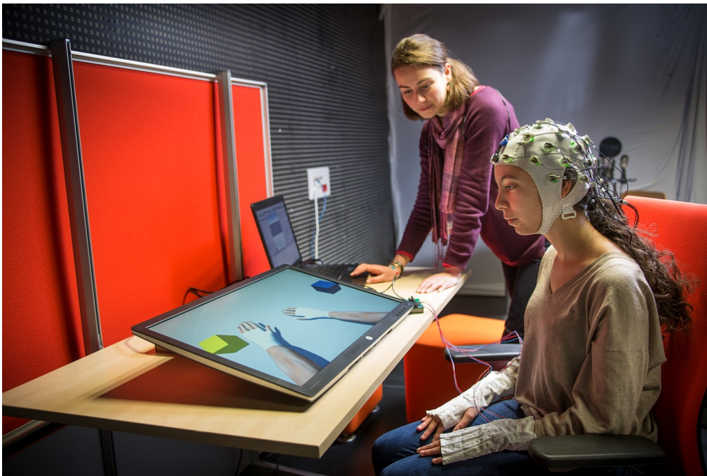
Figure 1: An example of a BCI system, that can detect in brain signals (here measured using electroencephalography (EEG)) whether the user is imagining or intending left or right hand movements, and shows 3D hands moving on screen accordingly, as feedback.
