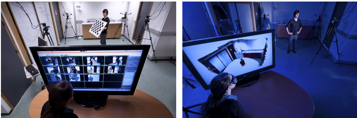
Figure 2. The mixed TOF-stereo multiple-camera system developed in collaboration with Samsung Electronics. Left: Geometric calibration of the camera system. Right: Live 3D display.
