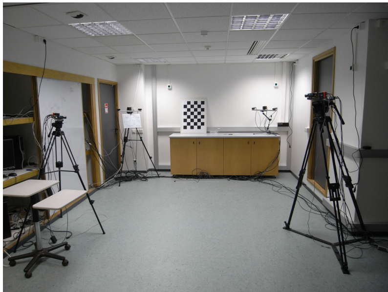
Figure 3. The mixed multi-camera system composed of four TOF-stereo sensor units.
