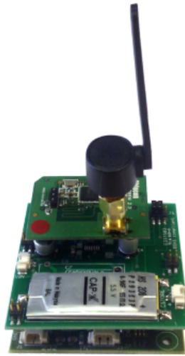
Figure 3. CAIRN's PowWow motherboard with radio and energy-harvesting boards connected
