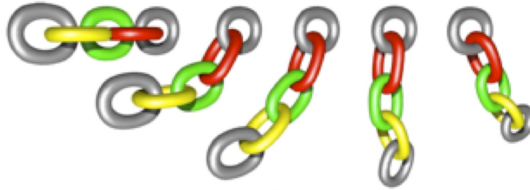
Figure 4. Animation of a chain combining a FEM model, a mass-spring model, a FFD grid, and a rigid body. This example is a perfect illustration of the flexibility of SOFA. Not only several algorithms for rigid or deformable bodies can be part of the same simulation, but they can also interact in a physically correct manner. No constraints between links were pre-defined, instead we relied on collision detection and stiff contact forces to handle the contacts. Using implicit integrator handling dynamically-created groups of interacting objects resulted in a stable simulation
