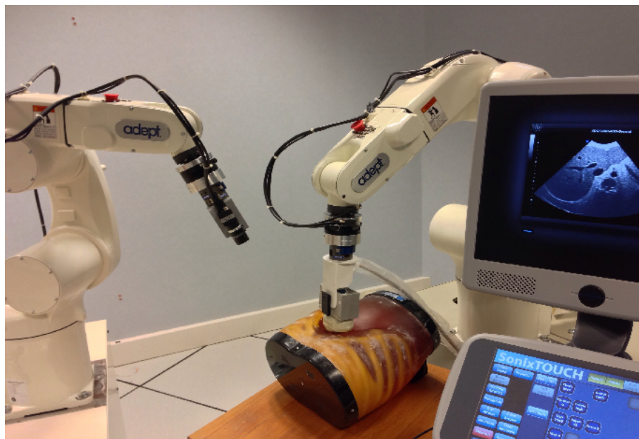
Figure 3. Lagadic medical robotics platforms. On the right Viper S850 robot arm equipped with a SonixTouch 3D ultrasound probe. On the left Viper S650 equipped with a tool changer that allows to attach a classical camera.
