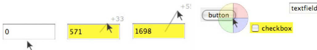
Figure 3. A numeric text field whose value can be set by a joystick-like interaction (left) and a semi-transparent menu to change the background color of Swing widgets (right)
