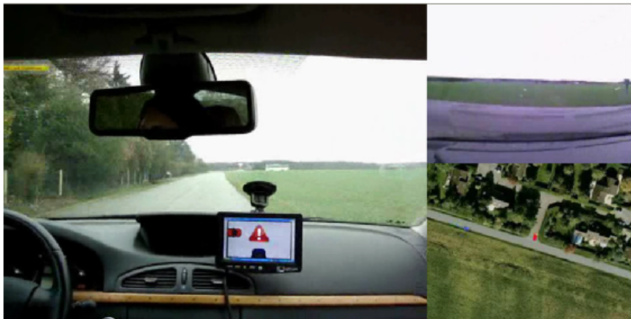
Figure 18. Online execution of the algorithm during the field trials: warning the driver of an upcoming collision with a vehicle on the left.
