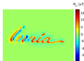
Figure 6. The Z-component of the magnetic field generated by the sample is measured by a SQUID microscope. The measure is performed 200\mu\text{m} above the sample.
