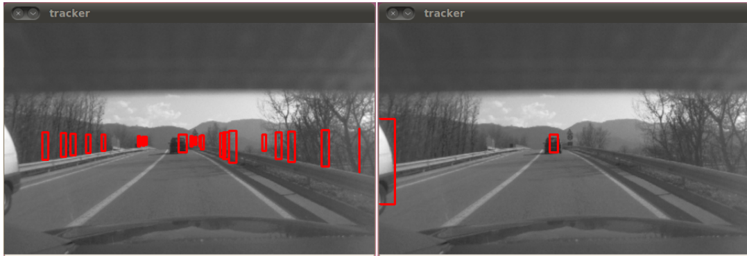
Figure 9. Tracking results of a car. Left, FCTA results without motion detection module activated. Right, same scenario but with motion detection module activated.
