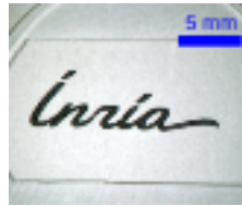
Figure 5. Inria’s logo were printed on a piece of paper. The ink of the letters “In” were magnetized along a direction D_1 . The ink of the letters “ria” were magnetized along another direction D_2 (almost orthogonal to D_1 ).
