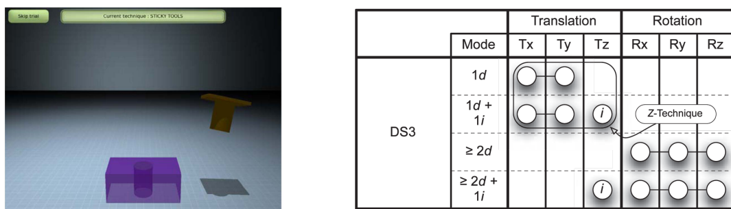
Figure 7. Screen capture of the peg-in-hole task used in the experiment (left). Description of the DS3 technique using the proposed taxonomy (right).
