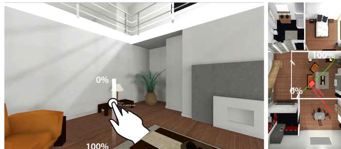
Figure 8. With the Drag'n Go method user can navigate in a 3D virtual environment with a multi-touch device. The movement speed is calculated using perspective based progression scale and it is let under the user's control.
