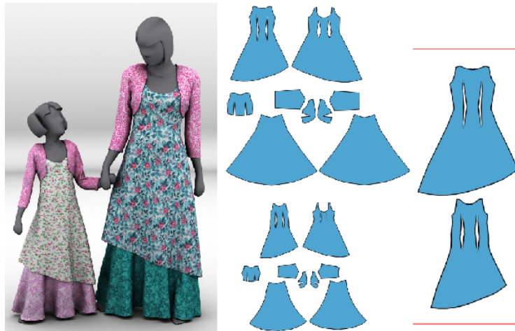
Figure 5. Design preserving garment transfer of a multi-layer outfit from a woman to a young girl. Middle: Automatically graded patterns shown to scale. Right: The zoomed-in source and target patterns for the back panel highlight the subtle changes in shape
