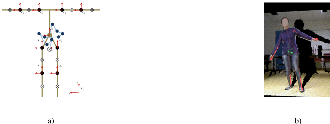
Figure 1. Center of mass estimation can be done using the statically equivalent serial chain. We assume a 9 rigid-link model (a) with spherical joints, capable of three dimensional movements. The SESC estimation can be performed in real time and is driven by joint angular measurements (b).
