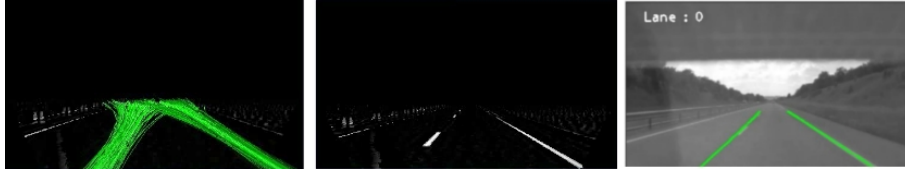
Figure 15. Vision-based tracking of the road markings. From left to right: particles generated by the particle filter, low level features extracted using the ridge filter, and estimated lane.
