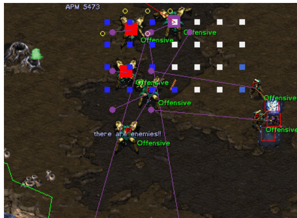
Figure 25. Units movement debugging output during a StarCraft game of the BroodwarBotQ bot. Considering the unit in the upper middle of the picture, white squares represent the highest probabilities of directions, while the darker the blue, the lower the probability to go there. The unit controller searches both to minimize collisions and stay in range of the enemy targets (bottom right).
