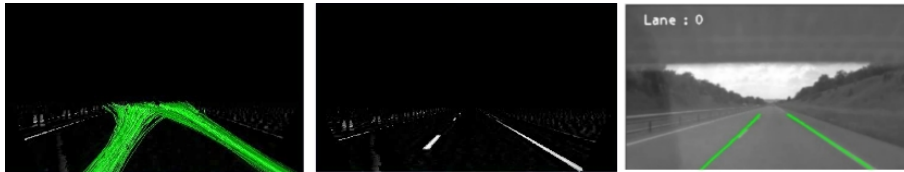
Figure 15. Vision-based tracking of the road markings. From left to right: particles generated by the particle filter, low level features extracted using the ridge filter, and estimated lane.
