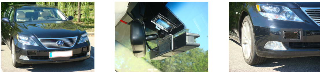
Figure 12. Lexus LS600h car equipped with two IBEO Lux lidars, a TYZX stereo camera, and a n Xsens MTi-G inertial sensor with GPS.
