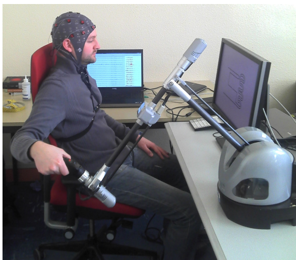
Figure 3. Proof-of-concept system combining Haptic and a Brain-Computer Interface (haptic guides are toggled based on a mental workload index computed by the BCI)
