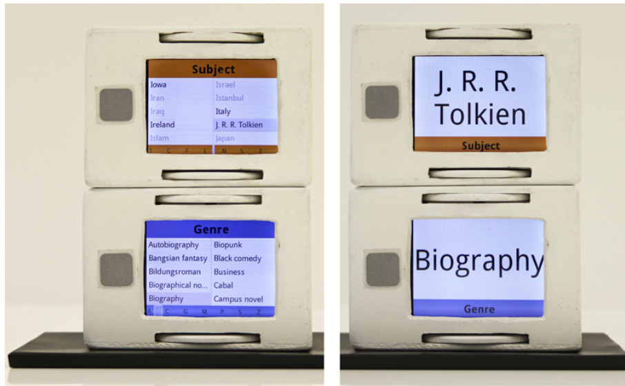
Figure 9. Four stackables. The left shows Stackables with their filter selection interface. The right two show the selected filters.
