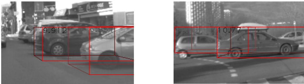
Figure 6. Car detection examples. The new weighting strategy allows to better detect the partially occluded objects.
