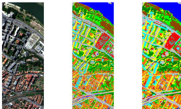
Figure 10. Center of Pavia image. (Left) Three-band color composite. (Middle) SVM classification map, overall classification accuracy = 94.9%. (Right) Classification map obtained using the proposed hierarchical approach, overall classification accuracy = 97.1%.
