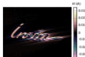
Figure 7. The field measured in Figure 6 is inverted, assuming that the sample is unidimensionally magnetized along the direction D_1 . The letters “In” are fairly well recovered while the rest of the letters is blurred (because the hypothesis about the direction of magnetization is false for “ria”).
