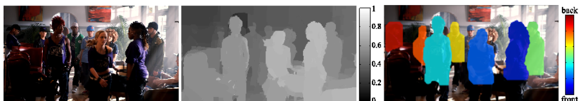
Figure 4. A sample frame extracted from the stereoscopic movie “StreetDance”: From left to right – left image from the stereo pair, disparity map computed from the stereo pair, layered segmentation of the image into 7 people. The front to back ordering is shown as a colour map, where “blue” denotes front and “red” denotes back. The cost function associated with our model is initialized using person detections, and incorporates disparity, pose, colour and motion cues. Note that the result shows accurate segmentation boundaries and also a reliable layer ordering of people.
