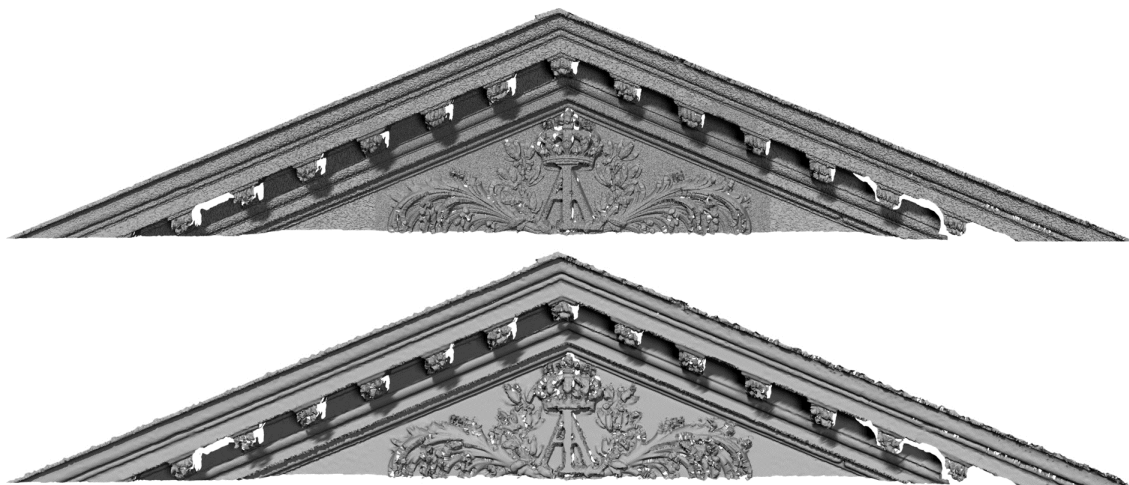
Figure 2. Similarity-based denoising. Top: input point set. Bottom: point set after denoising.
