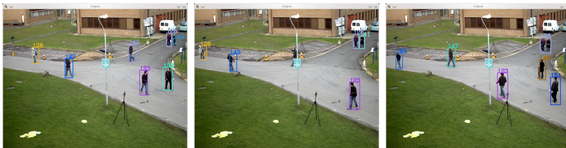
Figure 21. The global tracking challenge : correcting errors due to occlusions (ID 142 on the first frame becomes 147 on the last frame) and tracking people that are leaving the scene and reentering (ID 133 on the first frame becomes 151 on the last frame).
