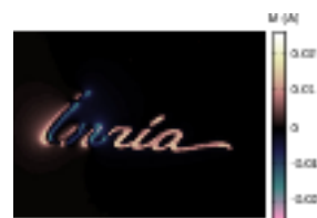
Figure 8. The field measured in Figure 6 is inverted, assuming that the sample is unidimensionally magnetized along the direction D_2 . The letters “ria” are fairly well recovered while the rest of the letters is blurred (because the hypothesis about the direction of magnetization is false for “In”).
