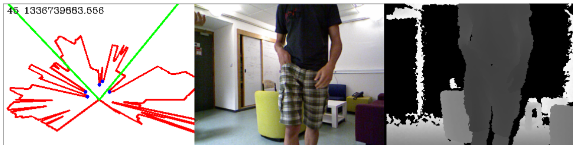
Figure 5. On the left image, one can see the telemeter range in red, the foot detection (blue spot) and the angle view from the Kinect (in green). the middle and right image represent RGB camera en depth view from the Kinect.
