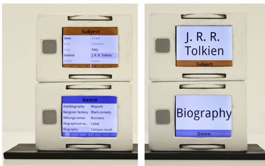
Figure 9. Four stackables. The left shows Stackables with their filter selection interface. The right two show the selected filters.
