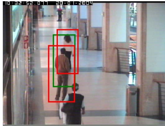
Figure 16. Illustration of the object detection correction for a Caviar video. The green bounding box is the output of the object detection process. The red bounding boxes are the results of the detection correction task.
