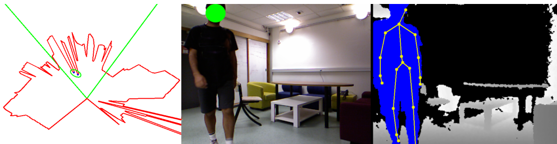
Figure 1. On the left image, one can see the telemeter range in red, the foot detection (blue spot) and the angle view from the Kinect (in green). the middle and right image represent RGB camera in depth view from the Kinect.
