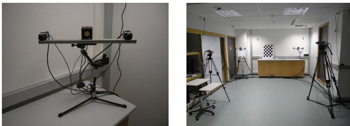
Figure 2. The MIXCAM laboratory is a multiple-camera multiple-PC hardware/software platform that combines high-resolution color (RGB) cameras with low-resolution time-of-flight (TOF) cameras. The cameras are arranged in “units”, where each unit is composed of two RGB cameras and one TOF camera (left image). Currently the system is composed of four such units (right image), or a total of eight RGB and four TOF cameras. Over years, in collaboration with 4D View Solutions, we have developed and maintained software packages for camera, multiple-camera, and cross-modal calibration, 3D reconstruction, multiple-camera stereo, TOF-stereo fusion, and image-based rendering.
