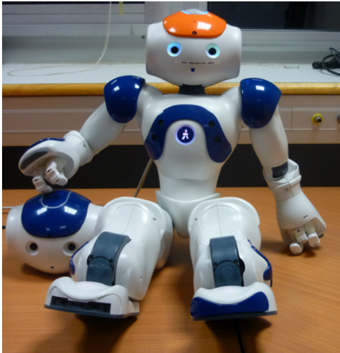
Figure 3. Left: The consumer humanoid robot NAO is equipped with a binocular-binaural head specially designed for human-humanoid interaction; Right: The binocular-binaural robot head POPEYE equipped with a four degrees of freedom stereo camera pair and with an acoustic dummy head.
