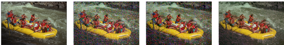
Figure 4. Image restoration demonstration on a severely corrupted image. The proposed method leads to a much better restoration quality compared to the standard BM3D method. From left to right: Ground-Truth, Noisy image, BM3D (20.46 dB), Proposed (22.25 dB).
