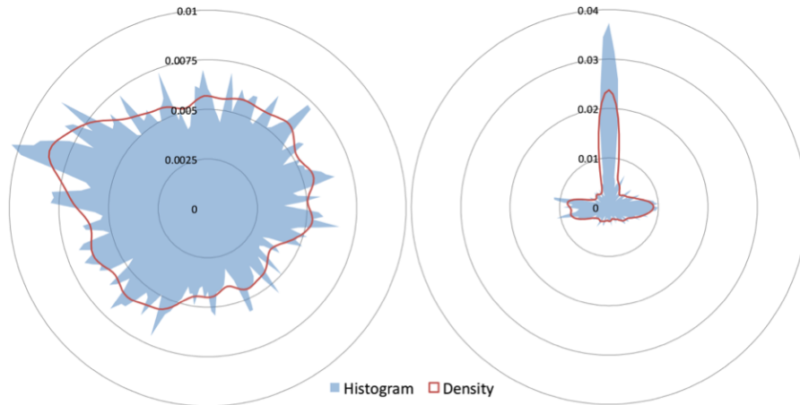
Figure 5. Distribution of traffic orientation for circle-shaped cells (left) and crossbow-shaped cells (right).
