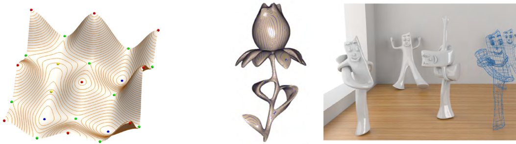
Figure 6. Illustration from [38](Left) showing our results on monotonic interpolation, and from [1](Right) with our G^1 interpolation surfaces for quad meshes.
