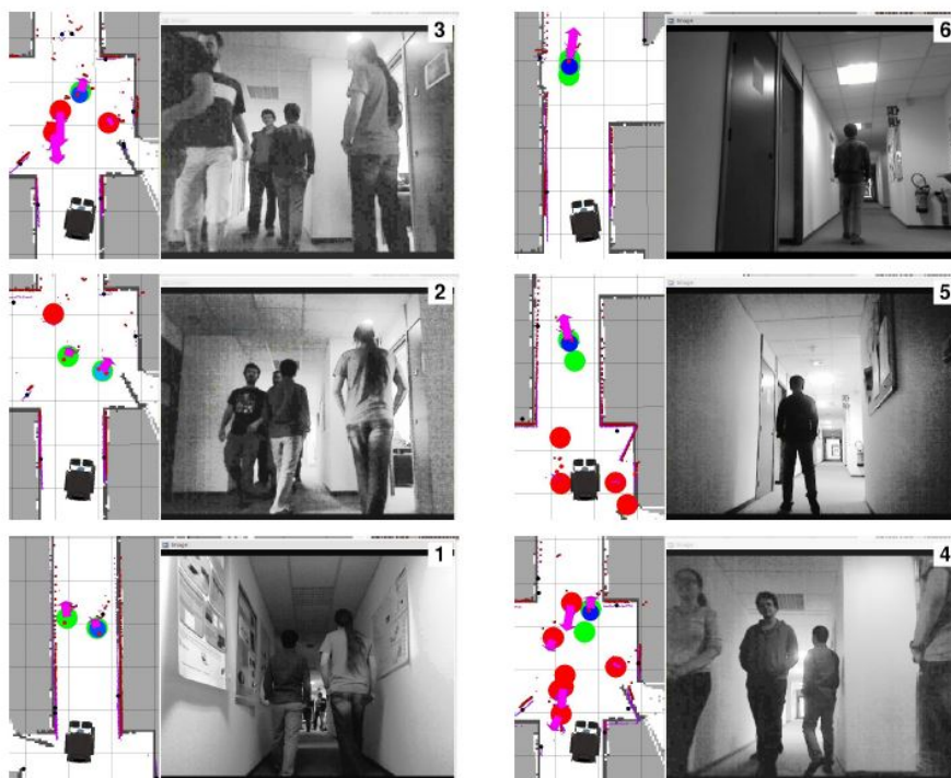
Figure 11. Switching navigation method between leader following and independent navigation. In image 1 the robot is engaged in leader following, while in the remaining it uses RiskRRT for the navigation.
