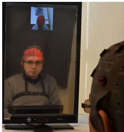
Figure 6. The Mind Mirror, a new real-time visualization tool of the user's own brain activity based on augmented reality.
