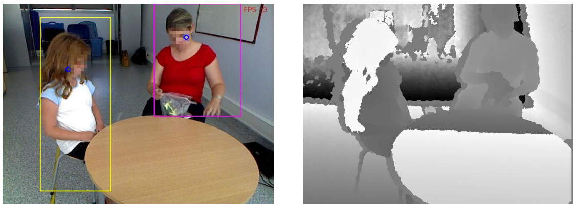
Figure 14. Result of head detection - good detection. The bounding box represents the person, the small blue circle represents the head center.
