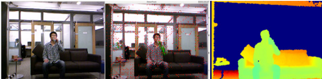
Figure 25. Visualization of MSR Daily Activity 3D data set (left) - video input frame, (center) - frame with detected trajectories (red - static points, green detected trajectories, (right) - corresponding depth map
