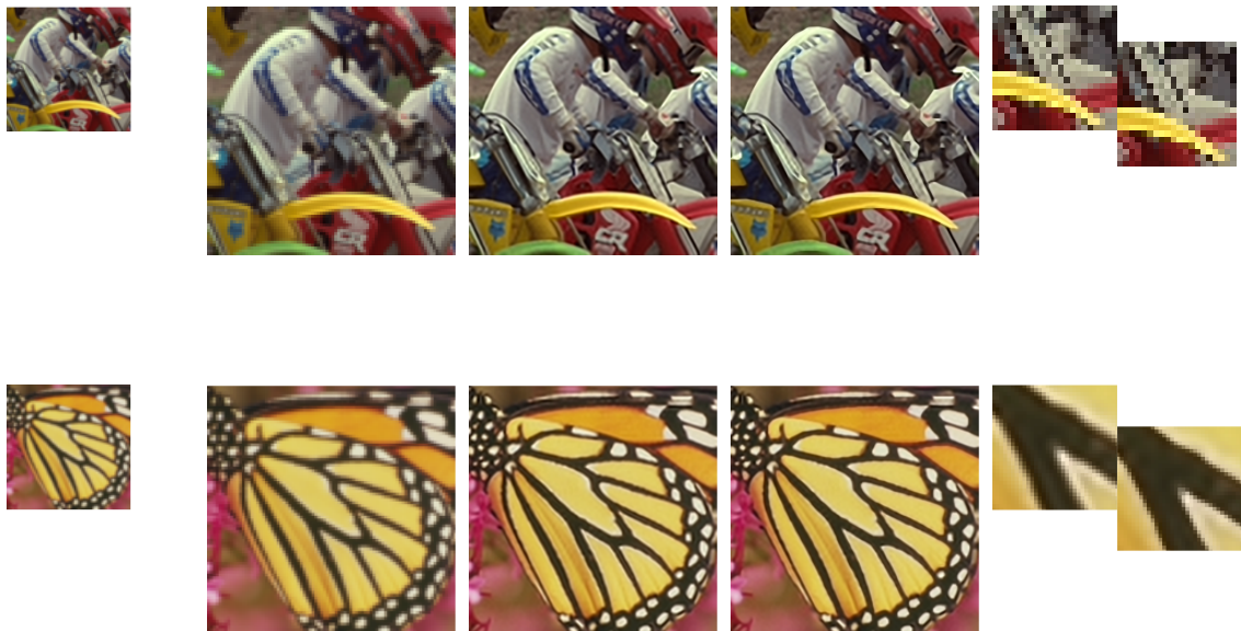
Figure 3. Comparison of SR results ( \times 3 ). (a) LR image; (b) Nearest-neighbor; (c) Sparse method without structure-based regularization; (d) SE-ASDS results. (e) Comparison between (c) and (d) on patches: edges of (d) are more contrasted than (c).
