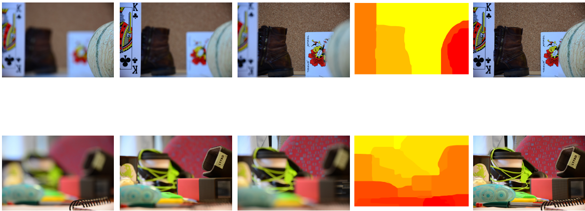
Figure 2. Three images of the focal stack (left); estimated depth map and image with extended focus (right). The focal stack images of the first and second rows have been captured with a Nikon 5200 camera.
