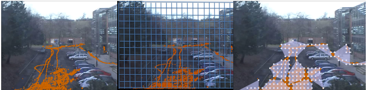
Figure 33. Example of Trajectories (left), Trajectories over the grid (center), that represents a given scale resolution, Zones discovering (right)
