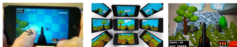
Figure 7. Touch (left), tilt (middle) and AR interaction techniques.
