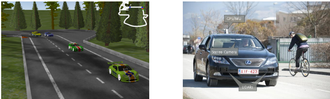
Figure 13. Experimental platforms: left) Our Torcs-based racing simulator; right) sensor-equipped Lexus vehicle.
