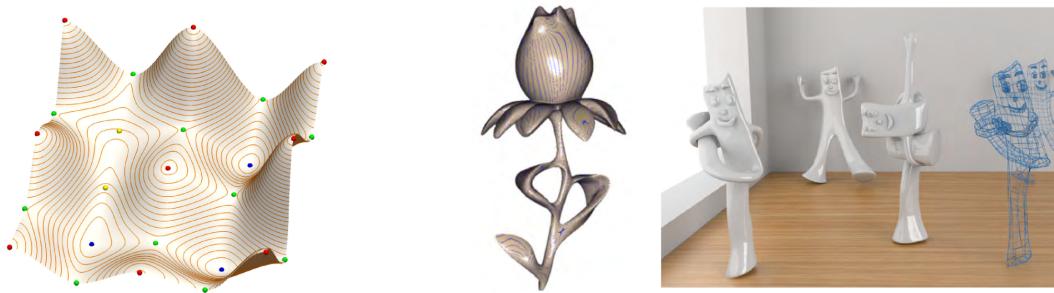
Figure 6. Illustration from [38](Left) showing our results on monotonic interpolation, and from [1](Right) with our G^1 interpolation surfaces for quad meshes.
