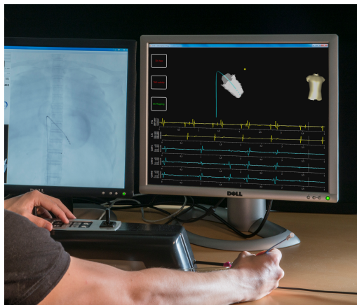
Figure 8. Training simulator for electrocardiology procedures
