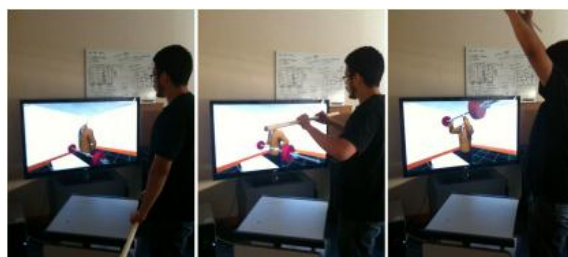
Figure 5. Weight discrimination task: the animation of the avatar showed a lifting effort according to the weight of the virtual dumbbell and the user has to rank the feedbacks from the lightest to the heaviest mass.
