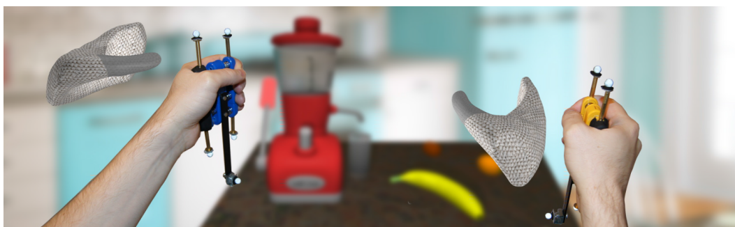
Figure 2. The Virtual Mitten : Visuo-haptic manipulation as enabled by our novel approach called the “Virtual Mitten”. Each hand holds an elastic device to control a virtual mitten (in grey) enabling the grasp of virtual objects.
