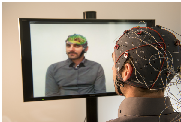
Figure 7. The Mind Mirror system : Visualization of brain activity in real-time using a mirror-based augmented reality setup and an EEG headset.
