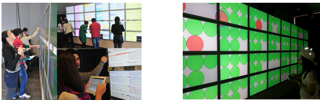
Figure 5. Left: Fine tuning the CHI 2013 conference schedule on the WILD display. Center: Classification task inspired by the CHI scheduling task conducted on the wall-sized display. Subjects must move misclassified red disks into containers (represented by the individual screens) of the same class. The class is represented by a very small letter at the center of each disk, forcing subjects to physically move in front of the display.
