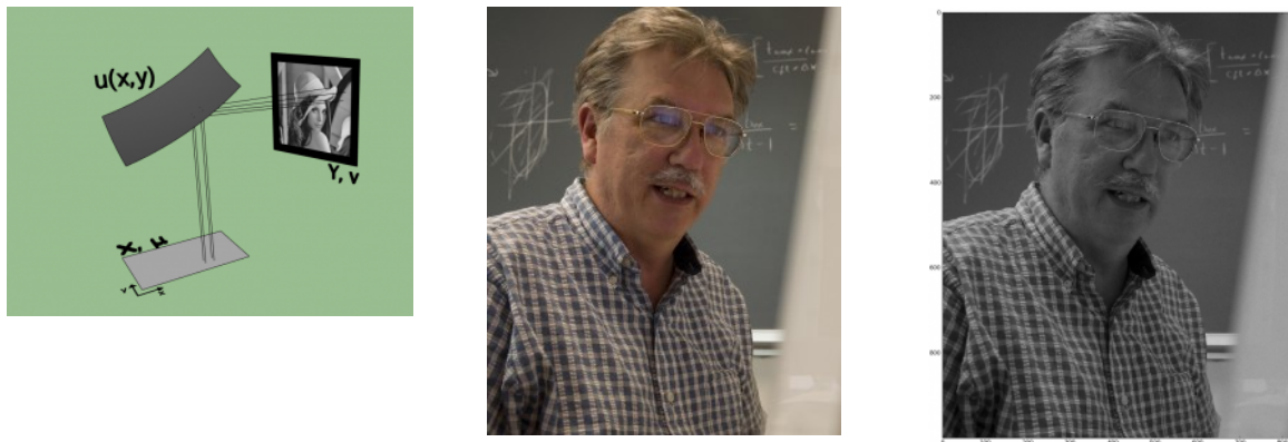
Figure 10. A constant source to a prescribed image (center). The reflector is computed (but not shown) and a resimulation using ray tracing shows the image reflected by the computed reflector.
