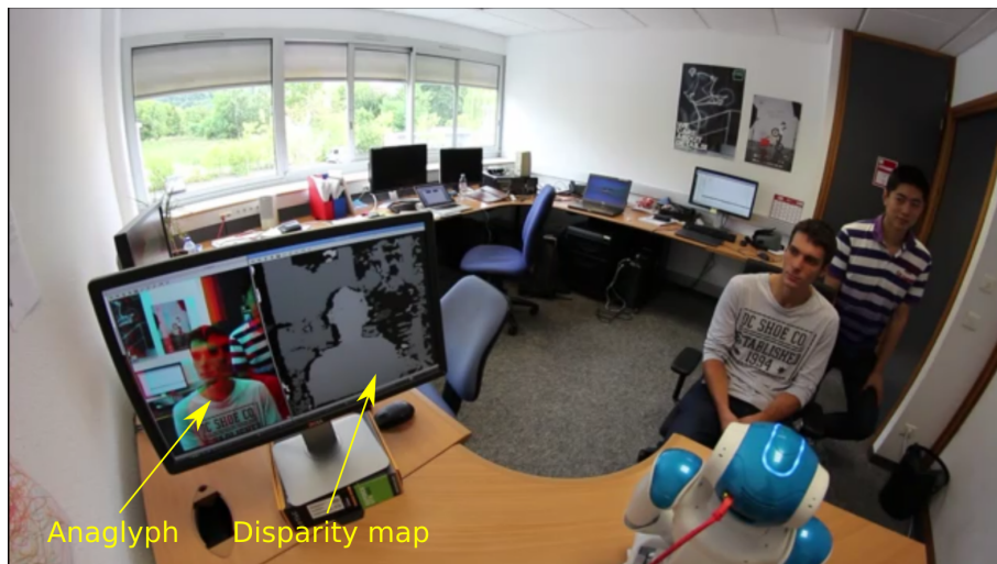
Figure 3. In collaboration with Aldebaran Robotics the team has developed a stereoscopic head for the humanoid robot NAO. Unlike the standard head that has a vertical pair of unsynchronized cameras (top-left), the new head has a horizontal pair of synchronized cameras (top-right). The latest prototype delivers VGA image pairs at 15 FPS. Based on the NAOLab library, we developed a stereo reconstruction method that delivers depth maps at 5 FPS (bottom).
