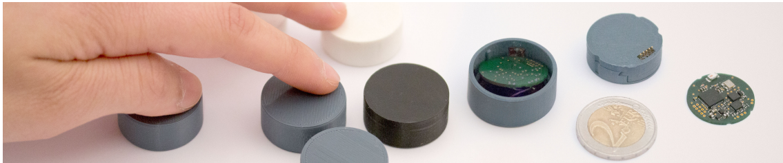
Figure 7. SmartTokens are small-sized tokens supporting touch and motion sensing, and wireless communication with a coordinator.
