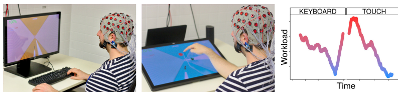
Figure 12. A keyboard (left) can be compared with a touch interface (middle) using a continuous measure of mental workload through electroencephalography (right).
