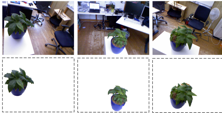
Figure 5. Three views of the PLANT dataset as processed by our method for multi-view silhouette extraction [3].
