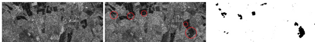
Figure 9. Change detection on a pair of 15 meter resolution XSAR images (first and second) obtained with a false discovery rate error metric based on the Cramer-von Mises statistic. The changes are highlighted with red circles (second), and the unsupervised detection result is reported in black (third).
