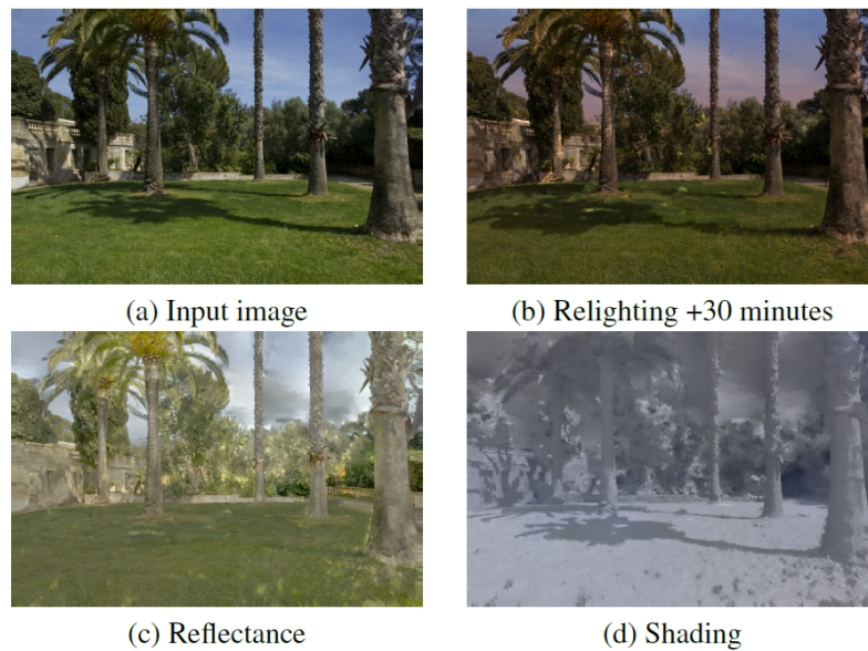
Figure 8. Our algorithm [2] decomposes outdoor images (a) into reflectance (c) and shading (d). This decomposition enables relighting of photographs by rendering new shadows in the shading layer (b).
