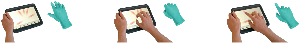
Figure 2. THING enables the control of 3D hand models (in blue) by sliding fingers along sliders arranged in a morphologically-consistent pattern on the tablet's screen.
