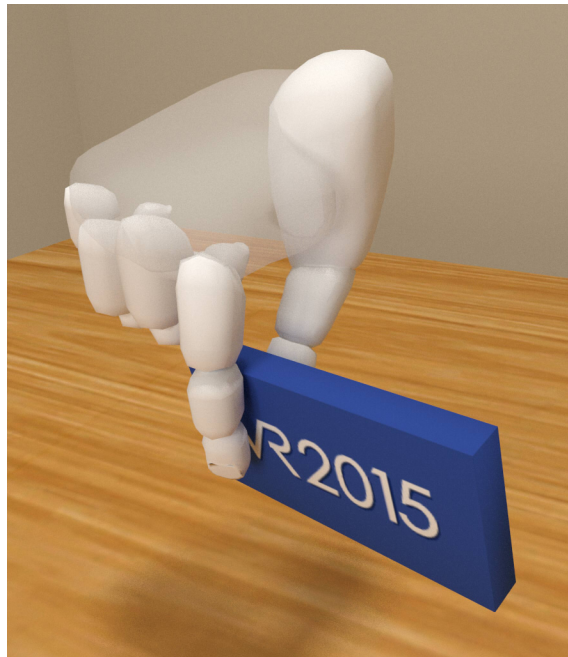
Figure 5. Interaction with deformable fingers generates many interconnected contact points which are expensive to solve with friction. Our approach aggregates contact constraints per phalanx with torsional friction. The subsequent increase in performance allows real time dexterous manipulation of virtual objects using soft fingers.
