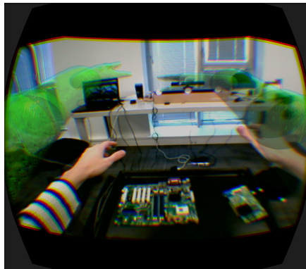
Figure 9. Remote collaborative maintenance using mixed reality.
