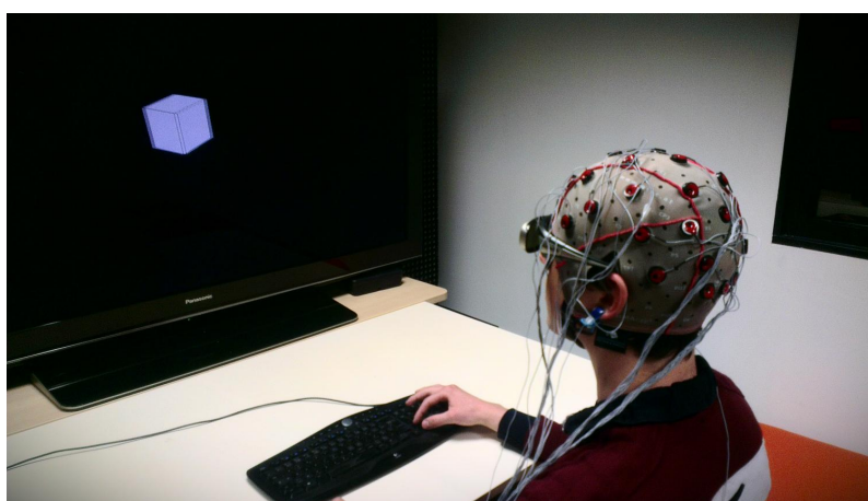
Figure 13. Setup of the experiment, with a subject being presented with stereoscopic images while his EEG signals are being recorded.
