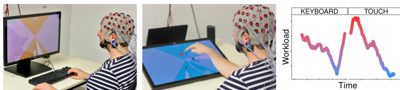
Figure 12. A keyboard (left) can be compared with a touch interface (middle) using a continuous measure of mental workload through electroencephalography (right).
