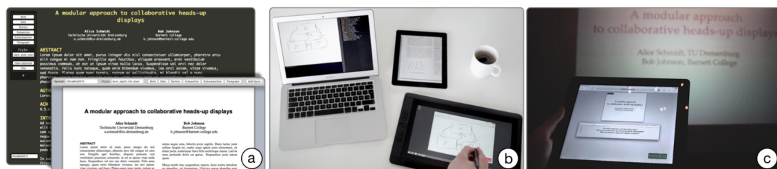
Figure 7. Sample uses of Webstrates: (a) Collaborative document authoring with different editors personalized at run-time; (b) Multiple devices used to sketch a figure (tablet 1), see it in a print preview (tablet 2), and adjust it in a graphics editor (laptop). (c) Distributed talk controlled remotely by a speaker with a separate interface for audience participation.
