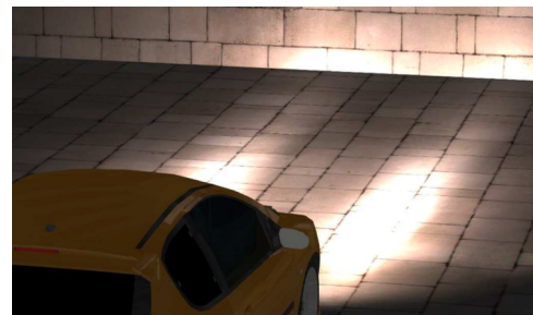
Figure 9. Our new light importance sampling technique estimates direct lighting interactively (7-9 fps) with only 200 samples per pixel that are distributed among the different images of the light field luminaire. The car headlights are represented by the same light field composed of 11 \times 9 images ( 256 \times 256 pixels).
