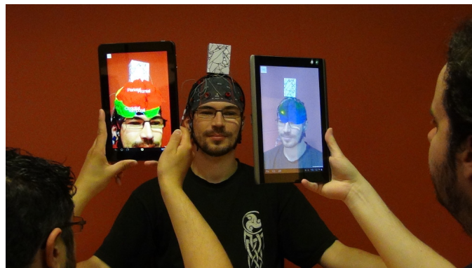
Figure 11. Our novel “Mind-Window” approach enables one or multiple users to visualize the brain activity of a person in real-time by using tablets and augmented reality. It proposes to see through the tablet a virtual brain model “as if the skull is transparent”. The display of the virtual brain is updated in real-time according to the real brain activity of the person which is measured thanks to an EEG headset.
