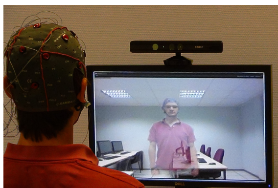
Figure 12. The “B-C-Invisibility power” enables users to become virtually invisible by performing mental tasks. Brain signals are extracted using EEG electrodes and analyzed within the BCI.
