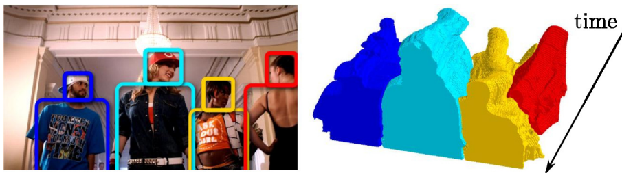
Figure 15. Results of our method applied to multi-person segmentation in a sample video from our database. Given an input video together with the tracks of object bounding boxes (left), our method finds pixel-wise segmentation for each object instance across video frames (right).
