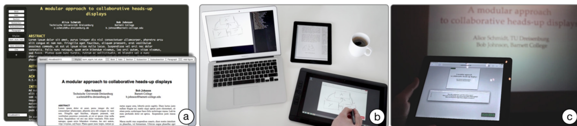
Figure 7. Sample uses of Webstrates: (a) Collaborative document authoring with different editors personalized at run-time; (b) Multiple devices used to sketch a figure (tablet 1), see it in a print preview (tablet 2), and adjust it in a graphics editor (laptop). (c) Distributed talk controlled remotely by a speaker with a separate interface for audience participation.
