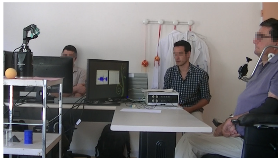
Figure 8. Principle of robot hand control through EMG signals; Setup description and upper arm positioning during EMG recordings.
